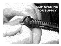
Starting at the rear of the tractor, attach the first clip to the frame inside the rear wheel well.
